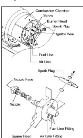
Figure 15. Removing Nozzle
